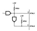
BOTH X1 AND X2 SHOULD BE DRIVEN. RESISTORS TO  $V_{CC}$  ARE NEEDED TO ENSURE  $V_{IH}$  = 3.8V IF TTL CIRCUITRY IS USED. THE MINIMUM HIGH AND THE MINIMUM LOW TIMES ARE 45%.
